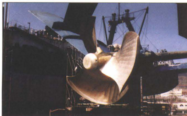
One of a pair of 1 m diameter CLT propeller units fitted to the 34 knot hydrofoil Barracuda . Owner Trasmediterranea now intends fitting CLTs to its other hydrofoils (p. 27)
