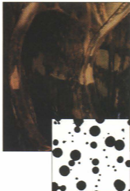
Coating at left is in "fair" condition, with 0.5% spot rusting, though there is coating breakdown on welds. Coating at right is in "poor" condition with >20% corrosion and discolorations
